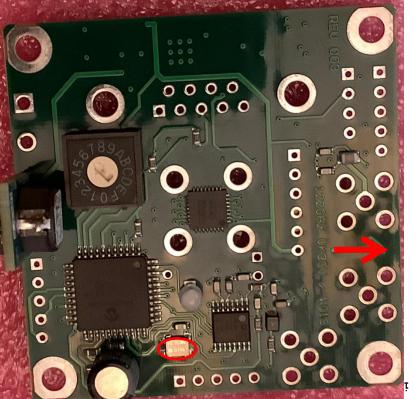
MAKE SURE ARROW IS HORIZONTAL for standard horizontal polarization!!!
