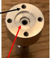
Adjust feed WG depth in combiner 1.2-1.8 mm above chip (max Rx sig, 2 step cavity)
