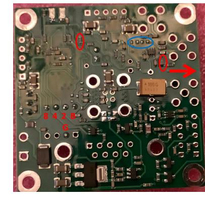
ICSP: PIC firmware programming port GPS: -, GND, - , - , 1PPS
