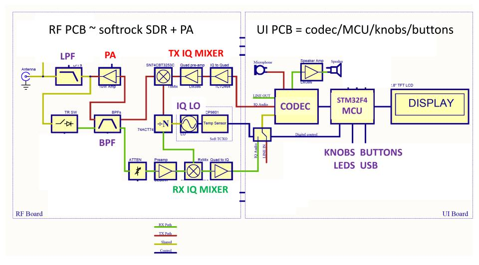
Quadrature Switching Detector Dir Conv / Low IF SDR (KX3 architecture is very similar)
