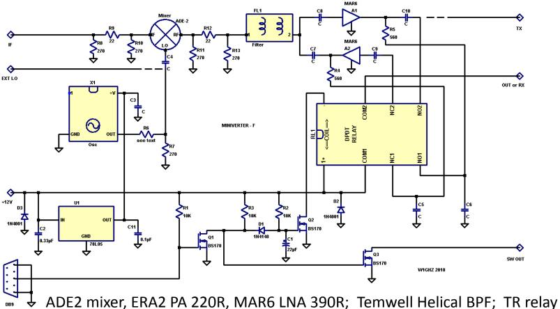
Conversion gain ~0/7 dB Rx/Tx P1dB ~10 dBm Rx NF ~2.3 dB, -7 IIP3 I modified PTT logic for T/R sequencing so that mcHF PTT out keys uwave xvtr, then uwave xvtr TxInhibit (817 style) activates miniverter TR relay Tx
