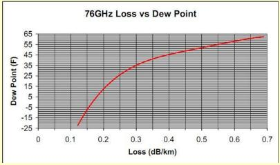
Free space Path loss:  $32.45 + 20\log(d) + 20\log(f)$ 250km = 178.5dB**Atmospherics** absorption @ 45 deg. 0.38dB/Km = 95dBTotal path loss 273.5dB Same as 23cm EME! In best case S/N would be - 29dB Time for new radio
