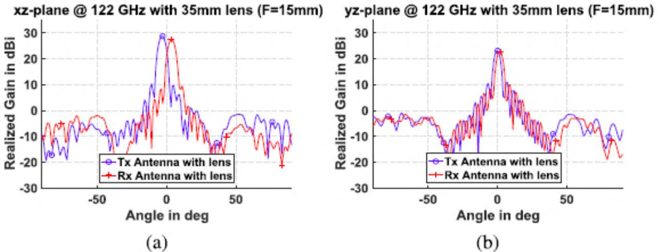
Plot (a) shows that the x axis separation is enough so that with the extra lens gain, the Rx peak is significantly displaced from the Tx peak. Plot (b) shows the effect of the y axis separation is proportionally less bad, but it still can be seen. This Tx / Rx pattern skew problem will only get worse with another 15 dB of dish reflector gain. For a 2 foot dish, it is estimated that the x axis Rx peak is anywhere between the Tx first null (most unfortunate!) and the Tx first side lobe.
