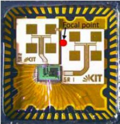
First, note that the ‘focal point’ for the following plots is the dot midway between the two antennas, **shown in the die photo at left**. The antennas are separated by ~3.0 mm in x and ~0.7mm in y.
