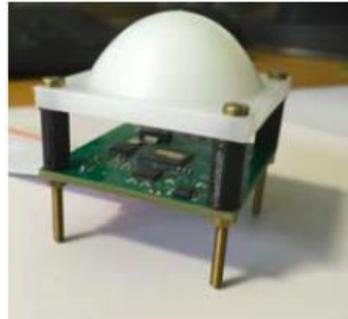
Next, in the following plots from [7], the gain has been increased to about 30 dBi with the addition of a **plastic lens in front of the package (center photo)**. As a result the beam width has narrowed enough to reveal the Tx / Rx beam skew issue caused by the antenna separation.
