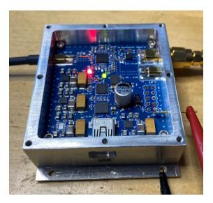
E band 80.832 GHz beacon with high performance frequency source.
