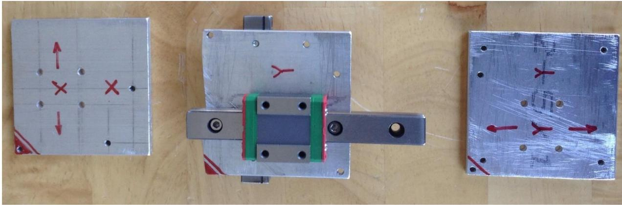
Assembled stage w/backlash springs on adjustable feed arm insert
